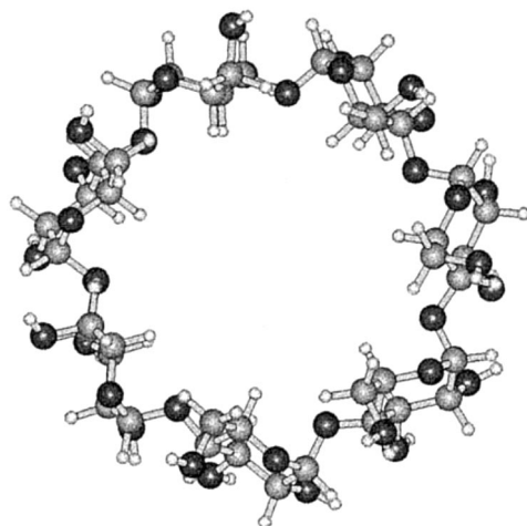
Fig. 1. Structure of \beta -cyclodextrin ( \beta -CD). Carbon atoms: light shading; oxygen: dark.
